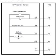
**NOTE:** Shielded cable must be used to connect all sensors, the ground or drain wire is to be connected at the controller end only.
